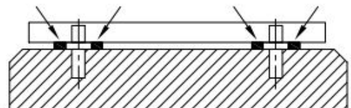
Fig.2 Foundation, baseplate and fitting the shims
