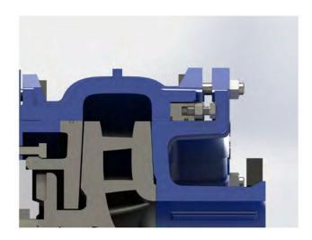
SSP-H pump series have major advantages to transfer fluid that has corrosive and abrasive properties. Even though these properties would have decrease pump performances in time, distance adjustment mechanisms on the SSP-H pump series can optimise the pump performances and improve service time.
