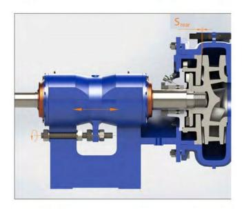
Stud bolts on bearing housing lead the movement of cartridge housing at SSP-H series HC/CR/CHC model pumps. Therefore distance between impeller and wear plate can be controlled. Rear clearance adjustment keep the pump performance up even wearing happens between the wear plate and the impeller.
