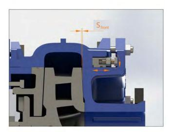
SSP-H series HC model pumps have front gap adjustment. Stop bolts in front of volute casing can set the gap between inlet port and impeller. Therefore negative effects of wearing optimise and service time of the pump improves. Besides that there is no need disassembly of volute casing and time is saved accordingly.
